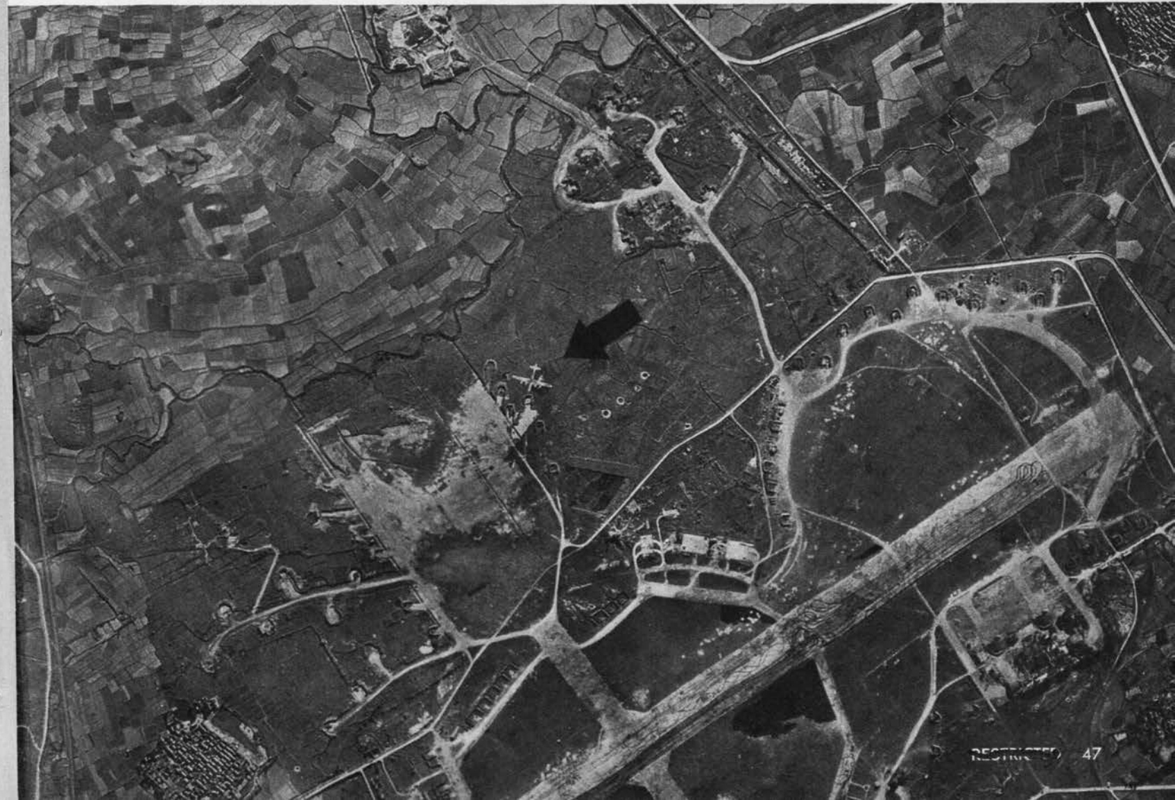
Airfield near Tokyo ( above ) shows a gravel-fill decoy. It casts no shadow and is not an accurate copy of any type, should not fool anybody.
